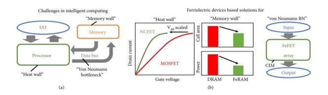
Schematics of (a) challenges faced by modern computers using von Neumann architecture and (b) solutions for "heat wall," "memory wall," and von Neumann bottleneck based on ferroelectric devices. Credit: *Intelligent Computing* (2022). DOI: 10.34133/2022/9859508
