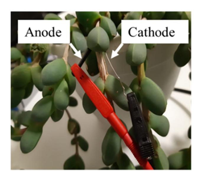
The ice plant succulent shown here can become a living solar cell and power a circuit using photosynthesis. Credit: *ACS Applied Materials & Interfaces* (2022). DOI: 10.1021/acsami.2c15123
