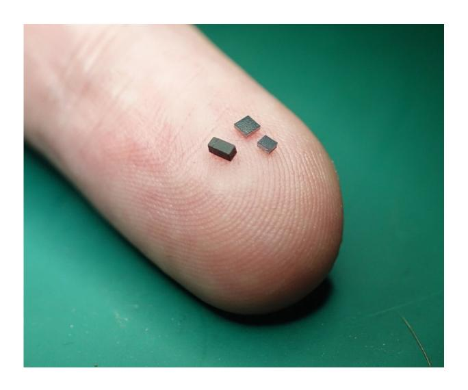
Image of the components of an avionics suite for a 10-mg "gnat robot" on a finger. They include a 2 mg gyroscope, 3 mg microprocessor, and a 1 mg visual optic flow sensor. Credit: Fuller, Yu & Talwekar.
