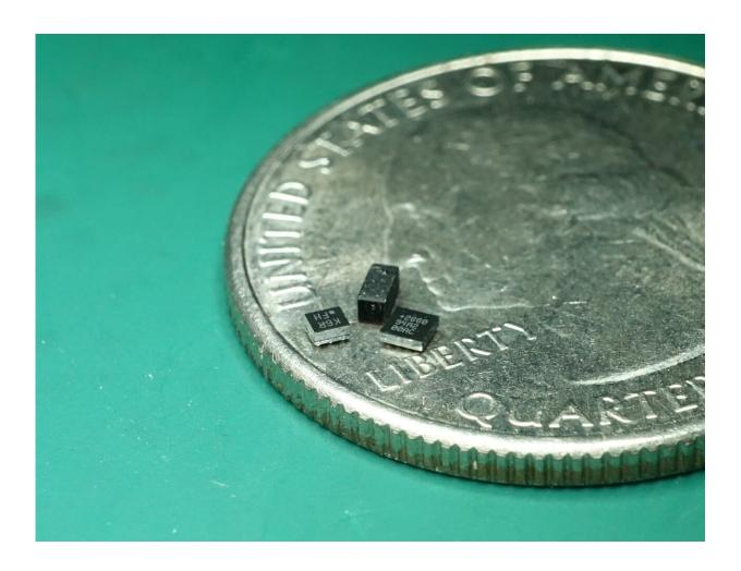
Images of the components of an avionics suite for a 10-mg "gnat robot" on a US Quarter Dollar coin. They include a 2 mg gyroscope, a 3 mg microprocessor, and a 1 mg visual optic flow sensor. Credit: Fuller.
