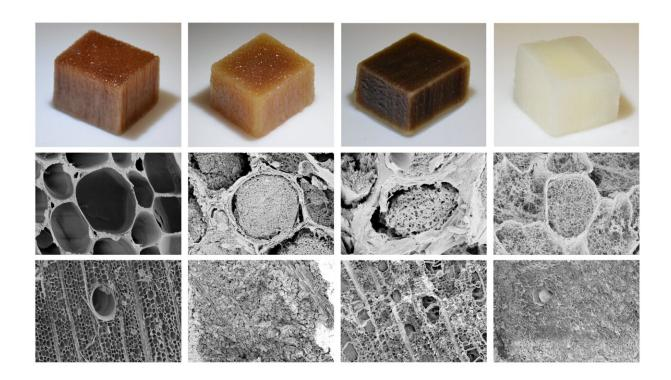
Highly porous nanoengineered wood for hydroelectricity harvesting was prepared through a one-step chemical treatment by immersing native wood (NW) into a water/NaOH mixture for 48 h at -6 °C. Credit: Yuanyuan Li
