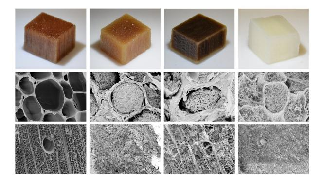
Highly porous nanoengineered wood for hydroelectricity harvesting was prepared through a one-step chemical treatment by immersing native wood (NW) into a water/NaOH mixture for 48 h at -6 °C. Credit: Yuanyuan Li
