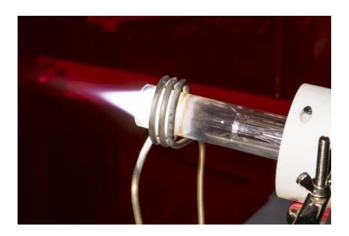
As part of research to evaluate CubeSats as airborne testbeds for technologies that are being developed for future generations of hypersonic vehicles, GTRI researchers developed this plasma source to produce high temperatures. Credit: Sean McNeil, GTRI
