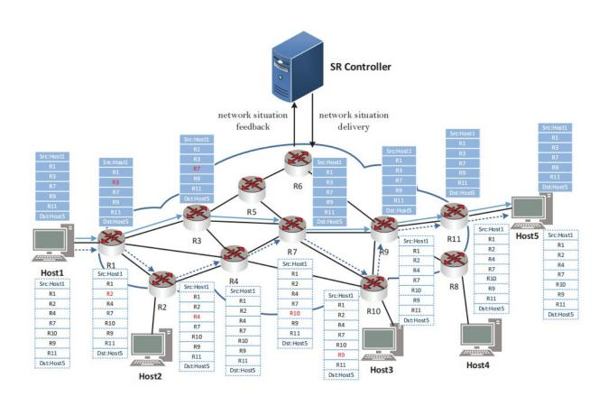
Case study illustrates the date transmission mechanism of diversion routing. Credit: Big Data Mining and Analytics, Tsinghua University Press
