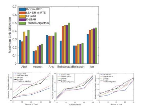
Graph showing load balancing performance of maximum bandwidth for algorithms in six selected topologies. Credit: Big Data Mining and Analytics, Tsinghua University Press
