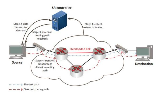
Diagram shows the total architecture of the intelligent routing scheme for traffic engineering. Credit: Big Data Mining and Analytics, Tsinghua University Press
