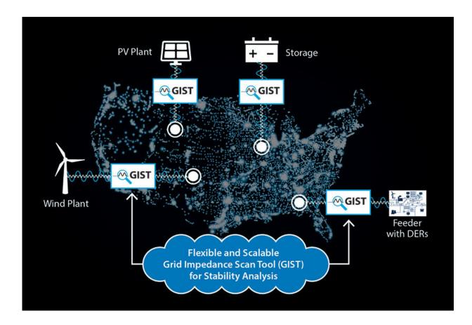
The Grid Impedance Scan Tool (GIST) sits between models of devices and the grid, allowing users to scan frequency dynamics and determine where unwanted stability issues could arise. Credit: National Renewable Energy Laboratory
