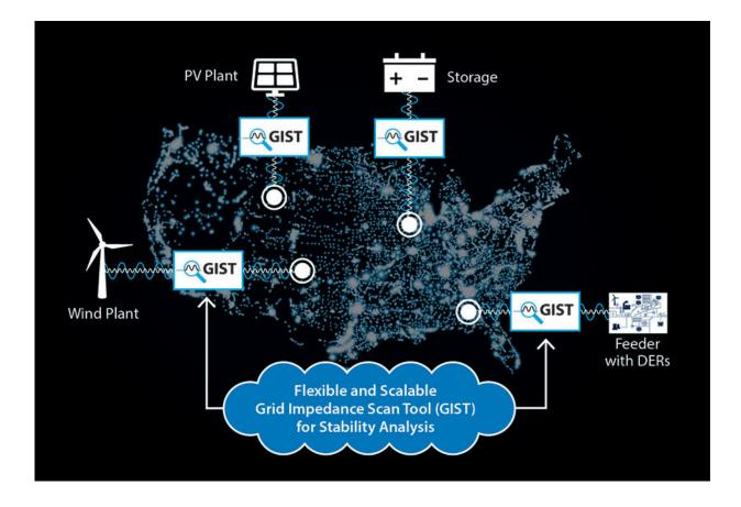
The Grid Impedance Scan Tool (GIST) sits between models of devices and the grid, allowing users to scan frequency dynamics and determine where unwanted stability issues could arise. Credit: National Renewable Energy Laboratory
