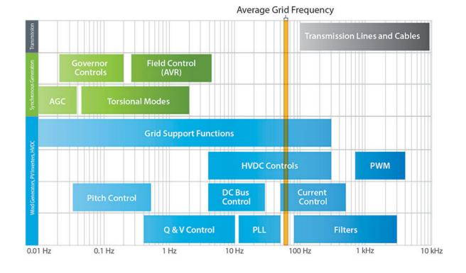
The frequency range of grid components expands well beyond the nominal operating frequency of 50 or 60 Hz. When grid controls and components oscillate outside of their expected range, serious stability issues can occur. Credit: Taylor Henry, NREL
