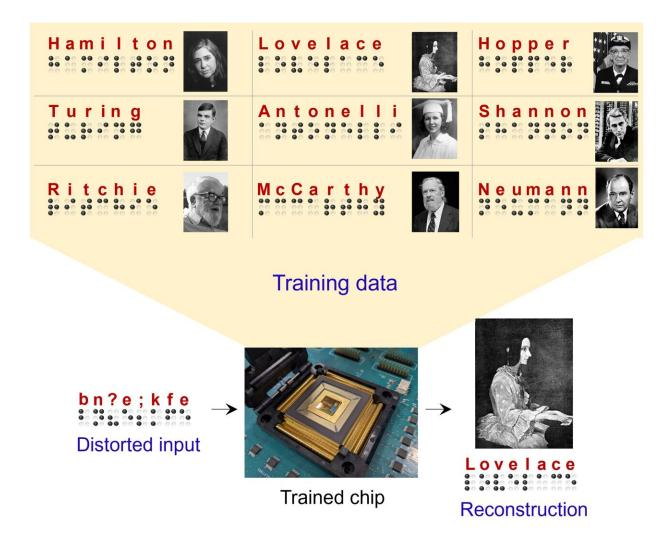
A chip consisting of memristor crossbars was trained using a local on-chip learning algorithm. The team demonstrated that their approach could accurately reconstruct Braille representations of nine famous computer scientists from highly distorted inputs. Credit: Yi et al.
