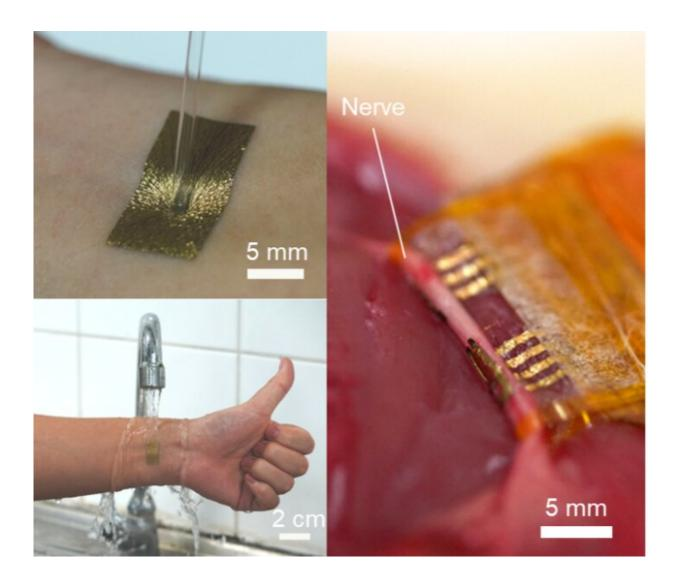
Images of ultrathin sensors forming a seamless and stable contact with human skin under dry and water-flush conditions and with a rat sciatic nerve. Credit: Jiang et al.
