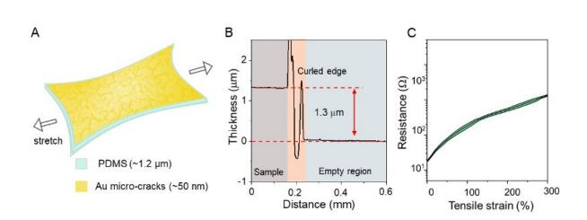
The ultrathin stretchable conductor based on PDMS and Au micro-cracks created by the researchers. (A) Structure illustration of the conductor. (B) Surface profile result of the conductor, showing a thickness of ~1.3  $\mu$ m. (C) The resistance change of the conductor under a series of strains. Credit: Jiang et al.
