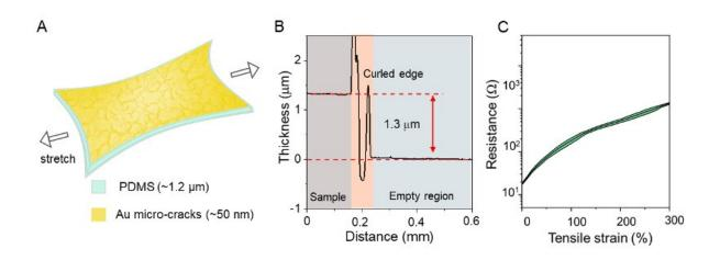
The ultrathin stretchable conductor based on PDMS and Au micro-cracks created by the researchers. (A) Structure illustration of the conductor. (B) Surface profile result of the conductor, showing a thickness of  $\sim 1.3 \, \mu m$ . (C) The resistance change of the conductor under a series of strains. Credit: Jiang et al.
