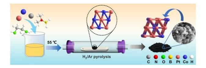
Highly ordered  $Pt_3Co$  nanoparticles were prepared by a two-step reduction strategy. The half wave potential of  $Pt_3Co/C$  reached 0.87 V, showing excellent ORR performance. Credit: Zhonghua Xiang, Beijing University of Chemical Technology
