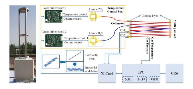
Photograph of the TDLAS sensor and schematic of the open-path TDLAS system used for measuring atmospheric  $H_2O$  and  $CO_2$  concentrations. Credit: Gu Mingsi
