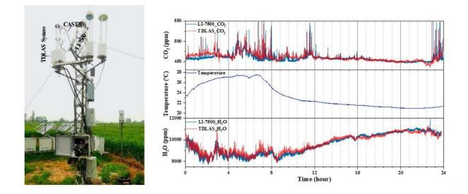
Photograph of the installation and comparison of the field measurements obtained using TDLAS and LI-7500 for 24 h. Credit: Gu Mingsi
