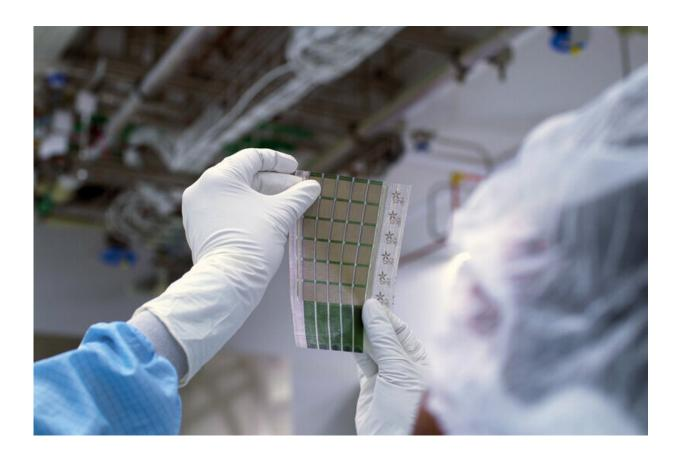
MIT researchers have developed a scalable fabrication technique to produce ultrathin, lightweight solar cells that can be stuck onto any surface. Credit: Melanie Gonick, MIT
