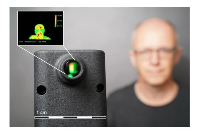
Portable system for displaying thermal images via power-saving OLED microdisplays. Credit: Fraunhofer FEP
