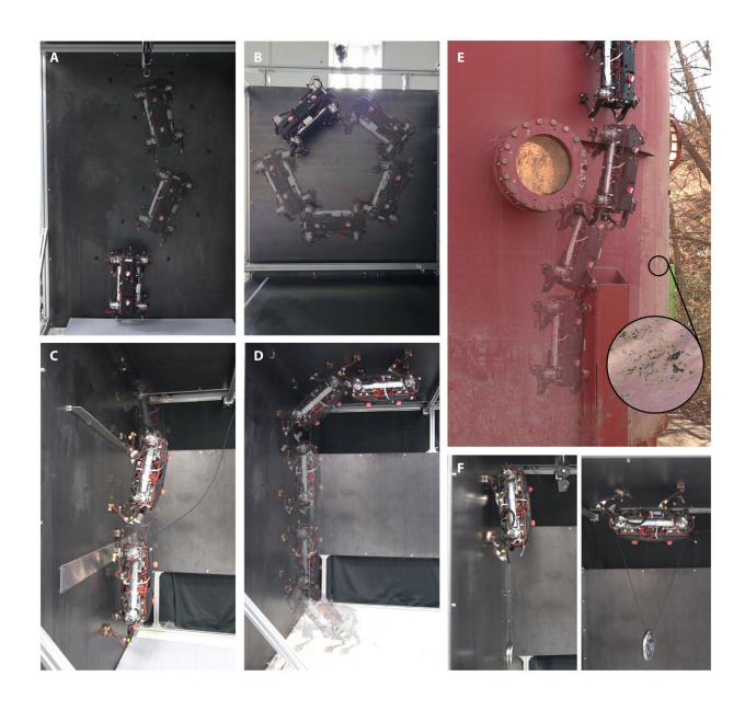
MARVEL performing various locomotion tasks. (A) Turning movement on a vertical wall. (B) Turning movement on a ceiling. (C) Traversing a gap (10 cm)
