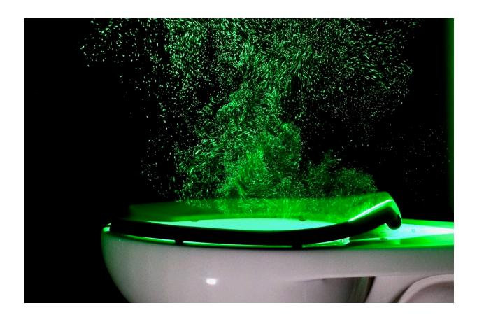
A powerful green laser helps visualize the aerosol plumes from a toilet while it's being flushed. Credit: John Crimaldi
