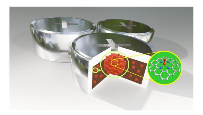
Going into detail: The porous catalyst (red balls) accomodates dense catalytically active zirconium sites (exemplified in the yellow circle) on its surface, thus improving the battery's chemical reactions associated to energy storage. Credit: HZDR / B. Schröder / M. Yu
