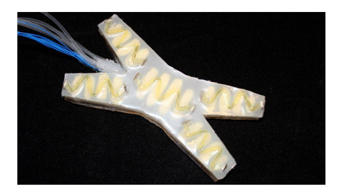
Researchers installed SHeaLDS—self-healing light guides for dynamic sensing—in a soft robot resembling a four-legged starfish and equipped with feedback control. After the researchers punctured one of its legs, the robot was able to detect the damage and self-heal the cuts. Credit: Cornell University
