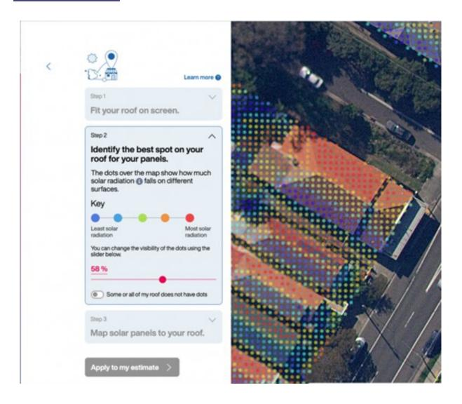
A premium version of SunSPOT shows users the best areas that solar panels could be placed, using red dots as an indicator. Credit: APVI
