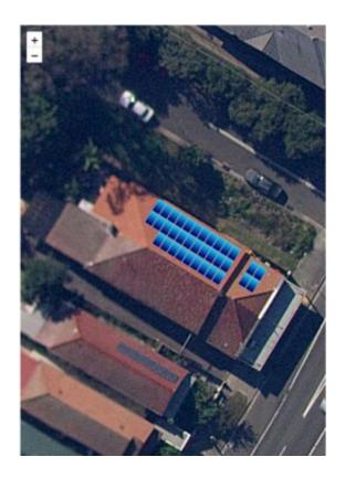
The SunSPOT tool helps users visualise where solar panels can be placed and how many might be possible, so they can run a cost-benefit analysis via the system. Credit: APVI
