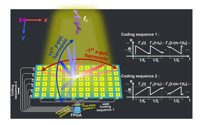
The space-frequency-polarization-division multiplexed wireless communication system, which can modulate different information on different carrier frequencies with different polarization states, and transmit them through different space channels independently and simultaneously. Credit: Science China Press
