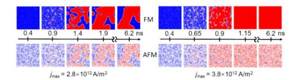
Micromagnetic simulations of the time-resolved and spatial-resolved SOT switching process. Credit: Wang et al
