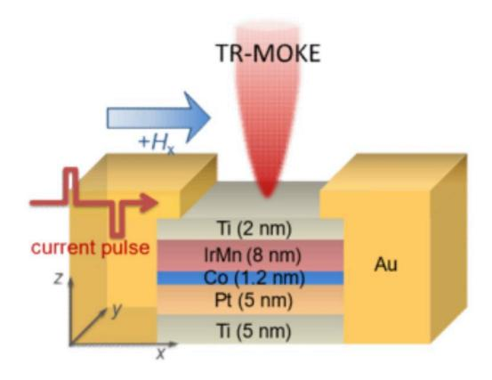
Concept of the experiment: In a stroboscopic time-resolved pump-probe experiment, the dynamic response of the magnetization is probed upon the application of short current pulses which induce so-called spin-orbit torques that lead to switching of the magnetization. Credit: Wang et al
