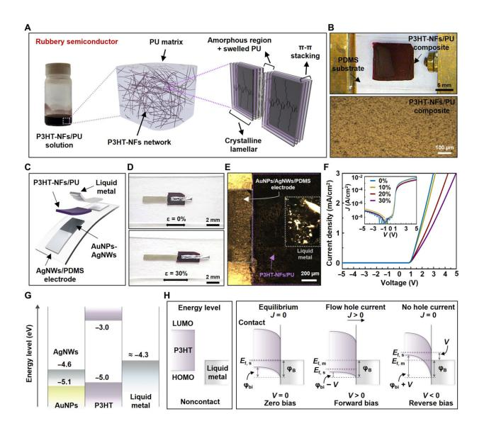
Fully rubbery Schottky diode. (A) An illustration of the morphology of the rubbery semiconductor composed of P3HT-NFs and PU. (B) An optical image
