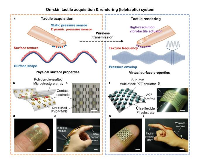
Ultra-flexible bimodal (UFB) tactile sensor and sub-mm tactile actuator array for telehaptic system. a Schematic of telehaptic system composed of tactile acquisition (left) and rendering (right). Physical surface properties including texture and shape are recorded by on-skin tactile sensor array and reproduced by
