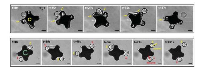
The researchers' microrobots use "physical intelligence" to exert control over nearby objects. By spinning and disrupting the alignment of the liquid crystal surrounding them, the robots can attract smaller particles to their edges, then precisely deposit them. Credit: University of Pennsylvania
