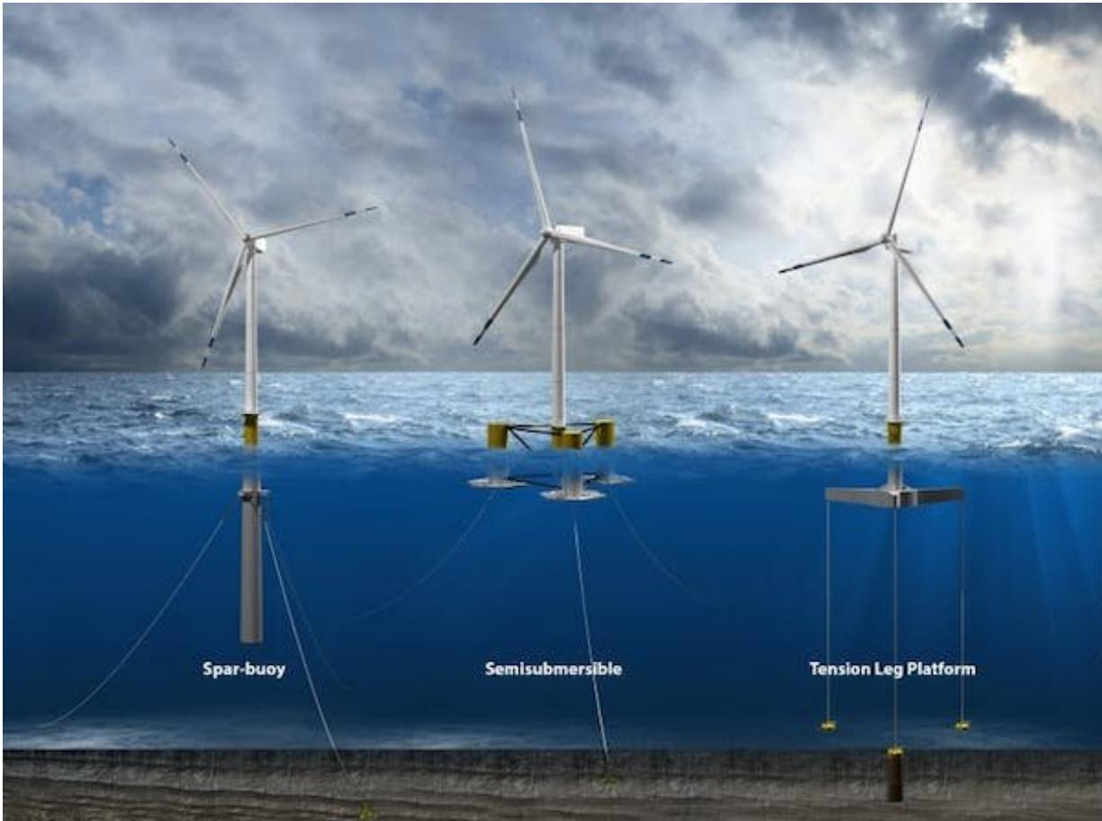
Three of the common types of floating wind turbine platform. Credit: [Josh Bauer/NREL](#)
