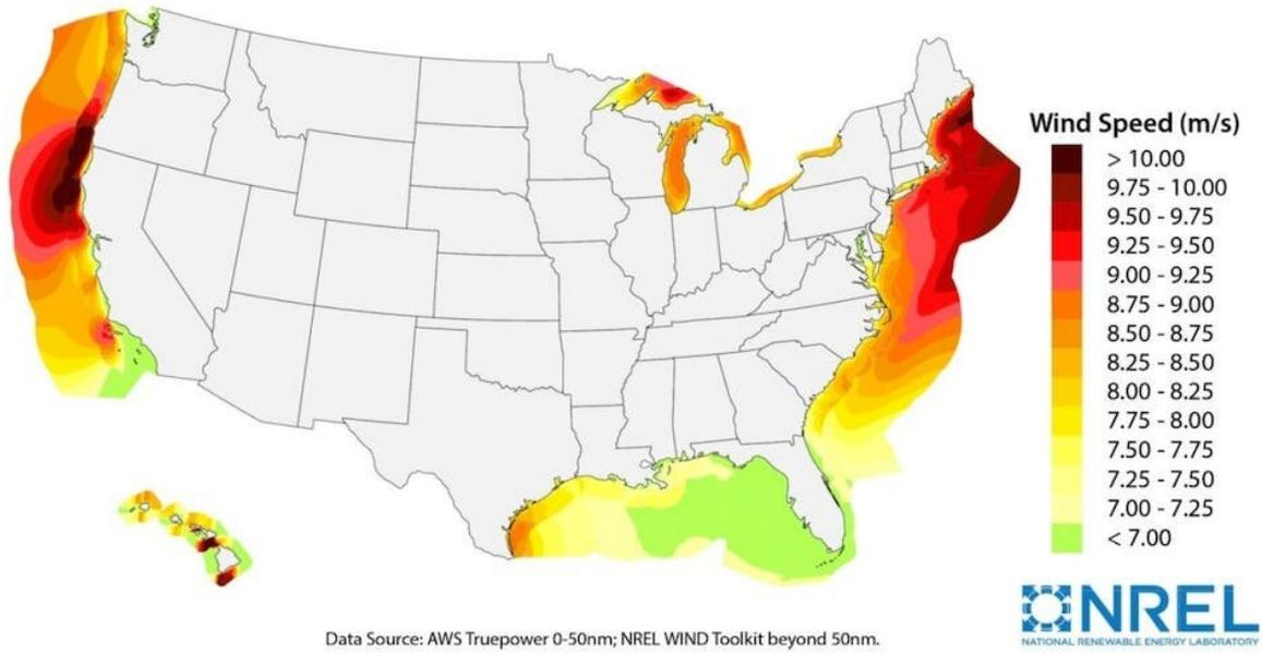
Some of the strongest offshore wind power potential in the U.S. is in areas where the water is too deep for fixed turbines, including off the West Coast. Credit: [NREL](#)
