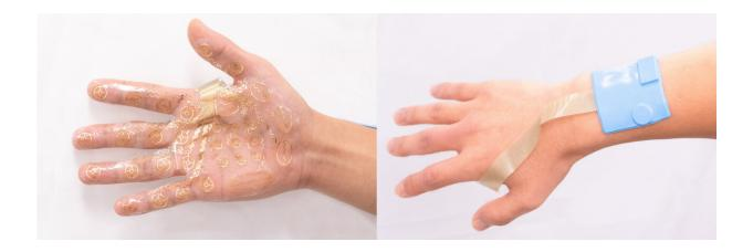
The wireless skin-integrated electrotactile system comprises two parts: a soft driver unit (right), attached to the forearm, and the hand patch (left). Credit: Dr Yu Xinge's research group / City University of Hong Kong
