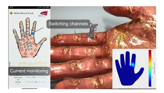
In an AR scenario, a virtual mouse hops forwards and rests briefly on each point of the hand. The hand patch, with hydrogel-based electrodes, has 32 electrotactile stimulation pixels on the palm side, allowing the threshold currents to be easily mapped for different users. Credit: City University of Hong Kong
