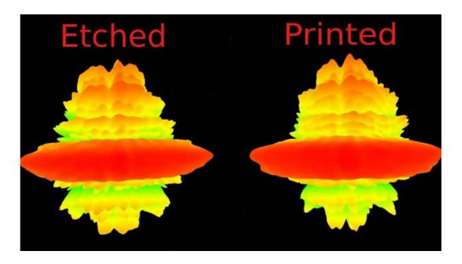
Picture of measured antennas' 3D surface plots. Credit: University of Sheffield
