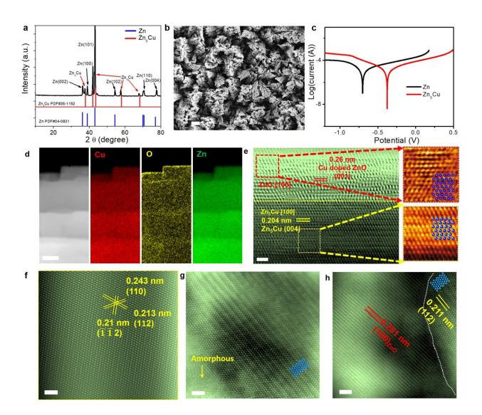
Structural characterizations of Zn-Cu anode. **a** XRD pattern. **b** SEM image of 3D Zn-Cu anodes. Scale bar: 10.0  $\mu$ m. **c** Tafel plots of Zn and Zn-Cu anodes. **d** EDS-mapping of Zn<sub>5</sub>Cu. Scale bar: 50 nm. **e** STEM image of the ZnO/Zn<sub>5</sub>Cu
