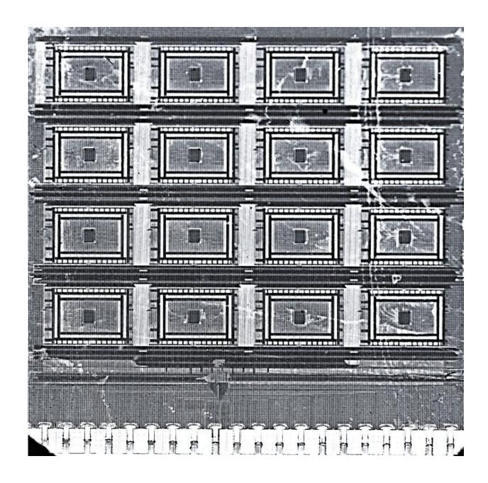
An optical microscopy image of the complete Bayesian machine. Credit: Damien Querlioz (CNRS/Univ. Paris-Saclay)
