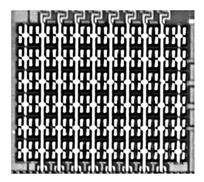
A zoomed-in optical microscopy image of the Bayesian machine on one of its 16 memristor arrays. Credit: Damien Querlioz (CNRS/Univ. Paris-Saclay)
