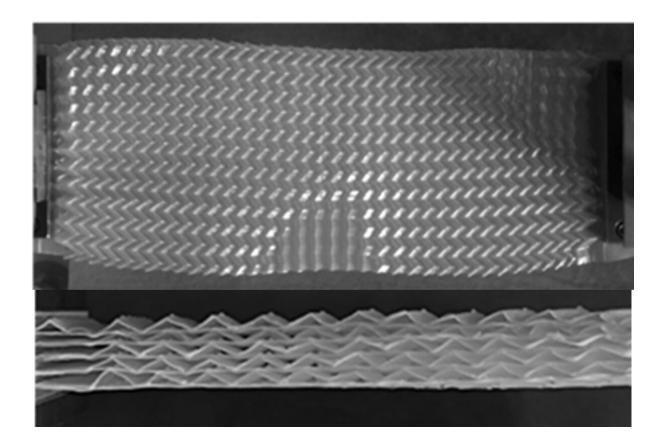
Above: Stiffness and shape change can be locally adjusted by patterning a film. Below: Stacking foils of different heights allows the creation of a programmable material. Credit: Fraunhofer ICT
