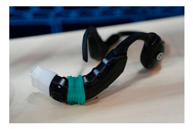
The OVR Technology ION 3 stand-alone wearable is on display at the OVR Technology booth during the CES tech show Thursday, Jan. 5, 2023, in Las Vegas. The ION 3 is a wearable device that delivers scents using cartridges, and the delivery system is synchronized with the content users are viewing in VR, AR, and mobile or desktop computing devices. Credit: AP Photo/John Locher
