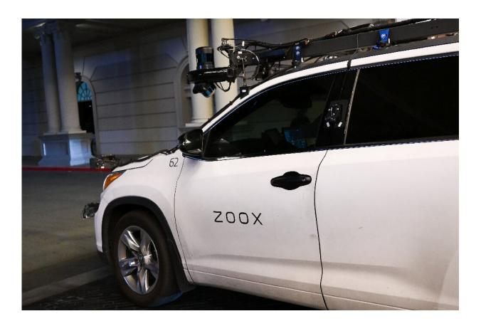
A Toyota sport-utility vehicle modified by Zoox, a subsidiary of Amazon.com, which combines radars, lidar, and cameras to test its software, drives on a road ahead.
