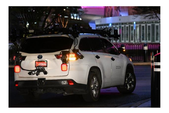
A Toyota sport-utility vehicle modified by Zoox, a subsidiary of Amazon.com, which combines radars, lidar, and cameras to test its software, drives on a road.
