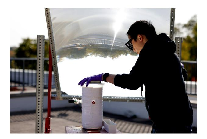
Peng Zhou uses a large lens to concentrate sunlight onto the water-splitting catalyst. Outdoors, the device was ten times more efficient than previous efforts at solar water splitting. Credit: Brenda Ahearn/Michigan Engineering, Communications and Marketing
