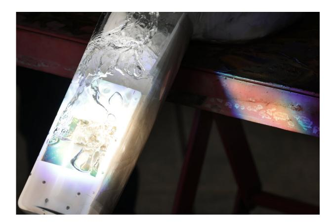
A close-up of the panel with the semiconductor catalyst and water inside. Bubbles of hydrogen and oxygen travel up the slope to be separated in the canister (maybe). Credit: Brenda Ahearn/Michigan Engineering, Communications and Marketing
