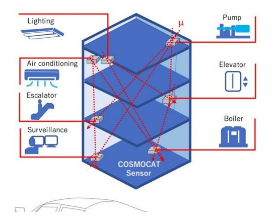
Some use cases for COSMOCAT. As the distance is limited due to the nature of the muon shower arriving at the ground, COSMOCAT is best suited for networks within small areas such as buildings. Offices, data centers and buildings that make use of smart devices, and even electric-car charging stations, are some possible application areas. Credit: ©2022 Hiroyuki Tanaka
