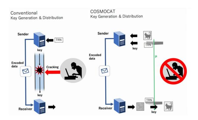
When both sender and receiver have identical random numbers, they can share encrypted data without the need to share a key to decode it. This prevents so-called man-in-the-middle attacks. With COSMOCAT, muons ( $\mu$ ) arriving at the sender and receiver at the same time provide the source of the random number. Provided the devices are synchronized, the receiver can know which muon signal relates to which incoming message and can decode it accordingly. Credit: ©2022 Hiroyuki Tanaka
