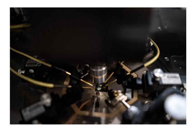
Memristors measured in a probe station. Credit: Technion Spokesperson Department.
