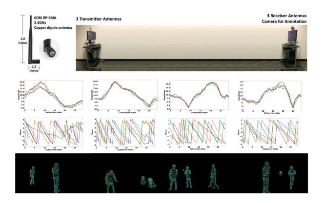
The first row illustrates the hardware setup. The second and third rows are the clips of amplitude and phase of the input WiFi signal. The fourth row contains the dense pose estimation of our algorithm from only the WiFi signal. Credit: *arXiv* (2023). DOI: 10.48550/arxiv.2301.00250
