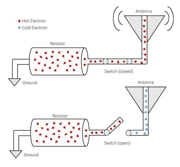
Electrons that naturally move around inside a room-temperature resistor affect electrons in a connected antenna, which causes the antenna to generate radio waves. Connecting and disconnecting the antenna produces the ones and zeros of a binary signal. Credit: Zerina Kapetanovic, <u>CC BY-ND</u>
