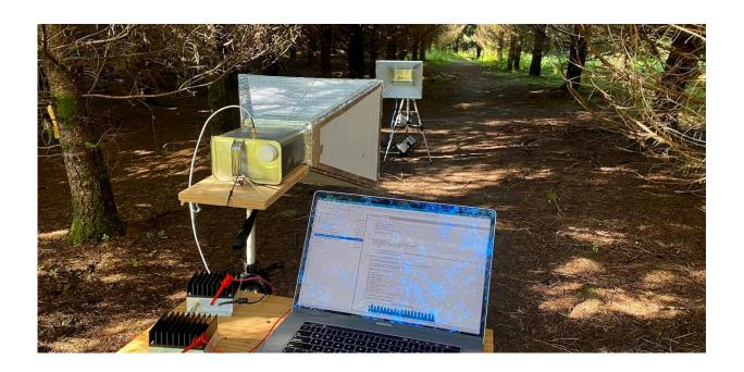
This experimental setup shows an ultra-low-power wireless communications device that could one day be used in tiny remote sensors. Credit: Zerina Kapetanovic, CC BY-ND
