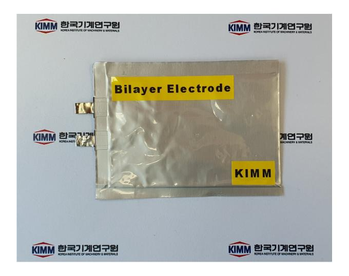
A bi-layer electrode battery in pouch form. Credit: Korea Institute of Machinery and Materials (KIMM)
