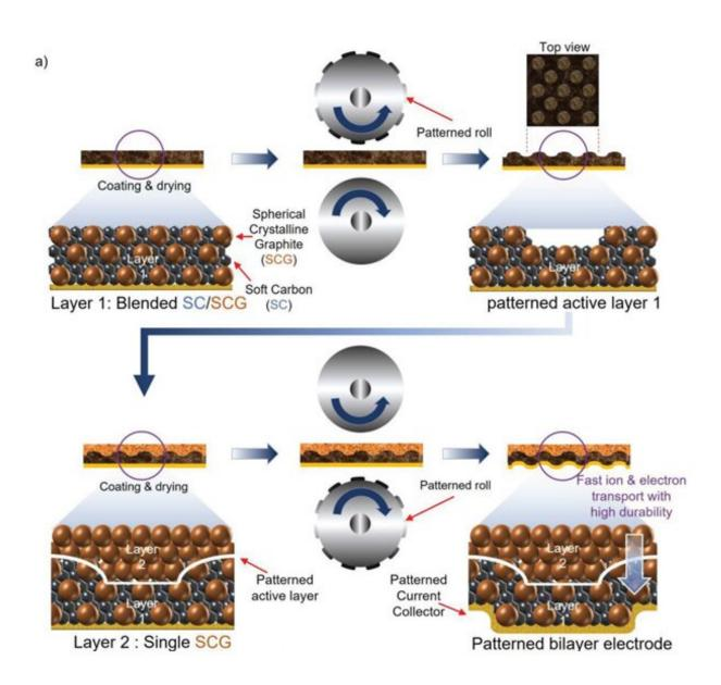
Electrode (anode) with a grooved, patterned bilayer structure. Credit: Korea
