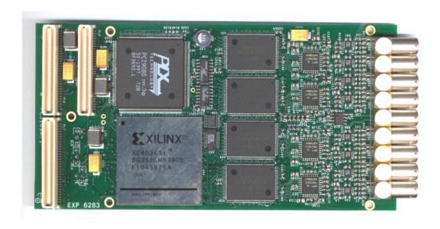
An FPGA-based readout card for the CMS tracker at CERN. Credit: CERN
