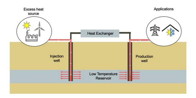
A conceptual schematic of the type of advanced geothermal energy storage system demonstrated in this study. Credit: Tugce Baser and *Renewable Energy*
