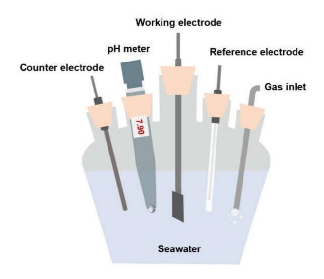
Schematic diagram of three-electrode configuration for seawater electrolysis. Note that the pH meter was placed 1.0 cm from the electrode surface to measure the pH of the bulk seawater near the working electrode. Credit: *Nature Energy*
