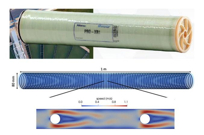
Hari Sitaraman and Ilenia Battiato have, for the first time, analyzed an entire reverse osmosis system, like the one seen here, with the greatest precision yet. With their simulations, the duo identified a new structural design that could improve the energy efficiency of these systems by a whopping 40%. Credit: Hari Sitaraman, NREL
