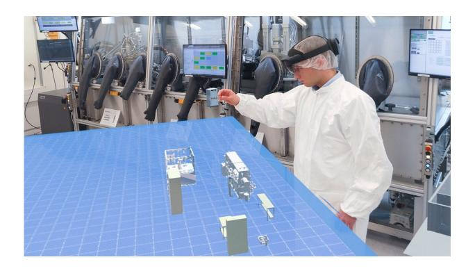
Layout planning with HoloLayouts in miniature mode. Credit: Fraunhofer IPA/Rainer Bez
