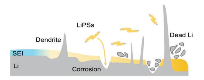
Challenges of Li metal anode in Li–S batteries. Both nonuniform Li stripping/plating and corrosion reactions with lithium polysulfides result in anode instability of Li–S batteries. *Energy Material Advances* (2023). DOI: 10.34133/energymatadv.0010
