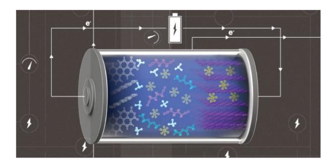
Illustration of the high-efficiency metal-free battery developed by KAUST researchers. Unlike conventional batteries, this battery combines an ammonium-cation-containing electrolyte with carbon-based electrodes. Credit: KAUST
