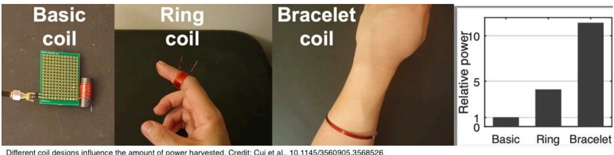
Different coil designs influence the amount of power harvested. Credit: Cui et al., 10.1145/3560905.3568526
