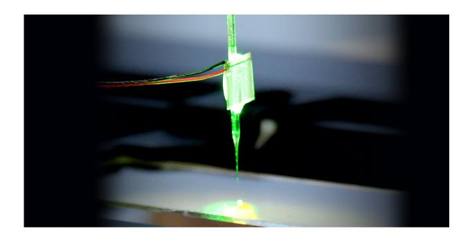
Using a glass needle made to oscillate with the assistance of ultrasound, liquids can be manipulated and particles can be trapped. Credit: ETH Zurich
