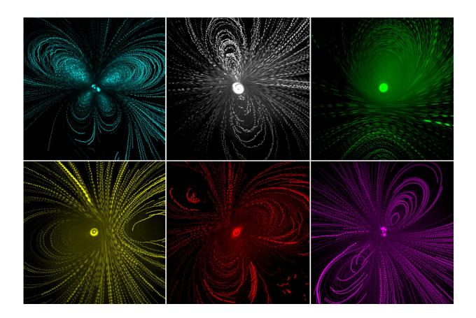
Various vortex patterns in liquids viewed from above and made visible by particles. The dot in the middle of each picture is the glass needle. Credit: ETH Zurich
