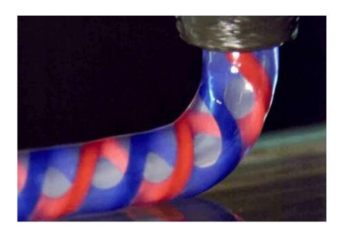
The inks are fed through a complex nozzle that allows multiple materials to be printed simultaneously. As the nozzle rotates and translates, the extruded inks form a filament with embedded helical features. Credit: Harvard University
