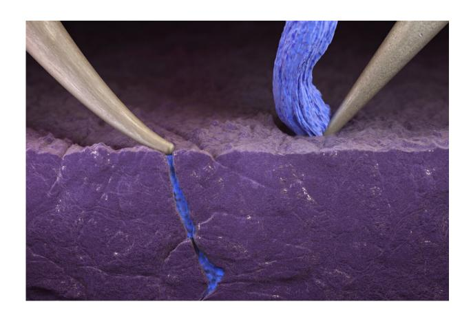
This artist's rendition shows one probe bending from applied pressure, causing a fracture in the solid electrolyte, which is filling with lithium. On the right, the probe is not pressing against the electrolyte and the lithium plates on the ceramic surface, as desired. Credit: Cube3D
