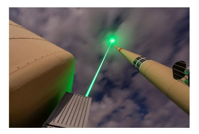
A laser on the top of a Swiss mountain, which managed to guide a lightning bolt for 50 meters.
