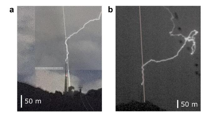
Lightning latches onto a laser, in the first time scientists have successfully diverted the path of a bolt with a beam.
