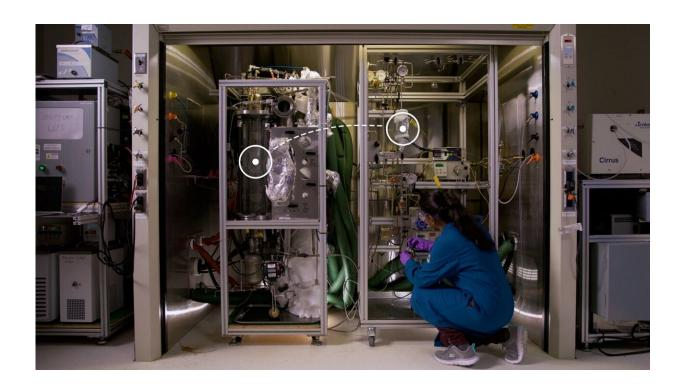
Taking up only as much space as a walk-in closet, a new carbon capture and conversion system is simple and efficient at removing carbon dioxide from gas that's rich with carbon dioxide. On the left of this walk-in fume hood, "smoke" moves through a cylindrical container where it makes contact with a carbon-capturing solvent. That solvent chemically binds to carbon dioxide and, on the right, is converted to methanol. Credit: Eric Francavilla | Pacific Northwest National Laboratory
